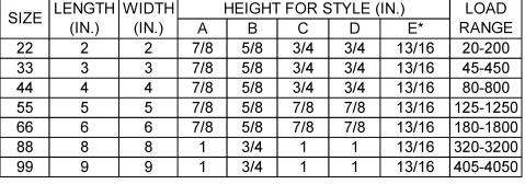
\*THIS HEIGHT BASED ON TWO PADS. FOR EACH ADDITIONAL PAD COMBINED, ADD 3/8"
